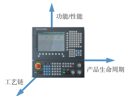
图2 开放式、智能化数控系统的多维度需求 Fig.2 Multi-dimensional requirements for open architecture and smart CNC system
